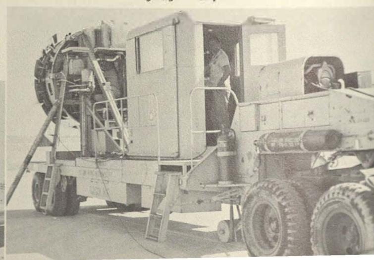
Running engine via portable test stand
